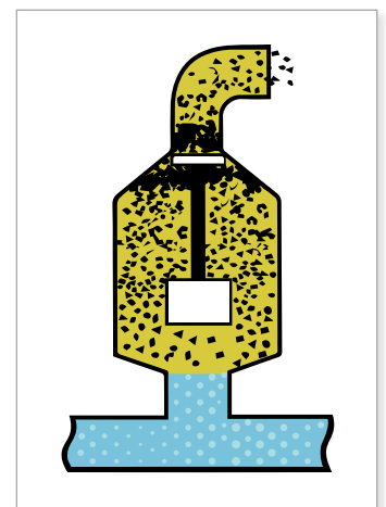
Negative flow rubbish 'bird nest' caught in valve. Blocked and/or leaking
